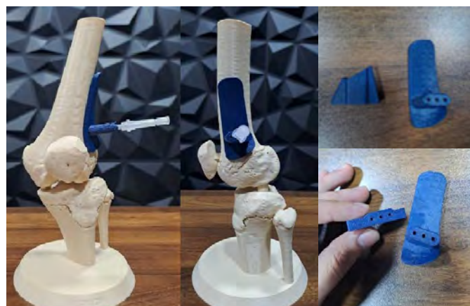
Figure 4. 3D printed guides on anatomical model of the patient
